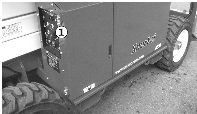
Figure 6.1.1 - Control Box Location, Ground Position
