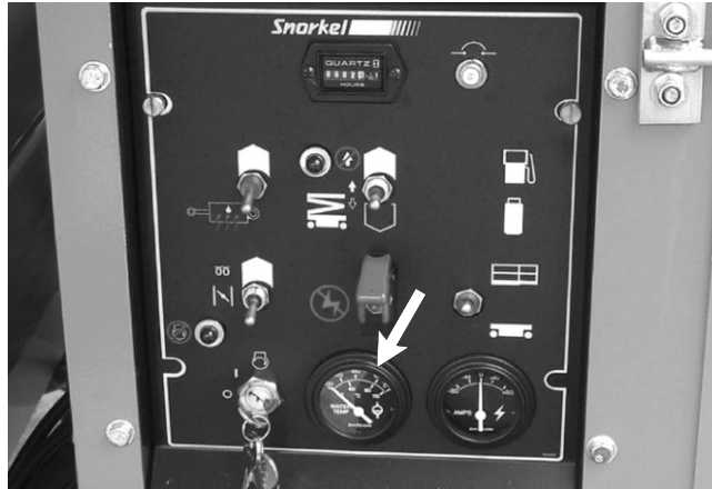
Figure 4.1 - Water Temperature Gauge
