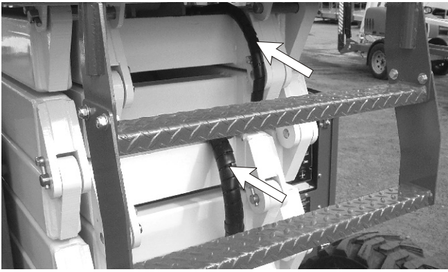
Figure 7.11 - Wiring Harness in the Scissor Stack
