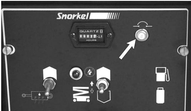
Figure 5.4 - Main Circuit Breaker
