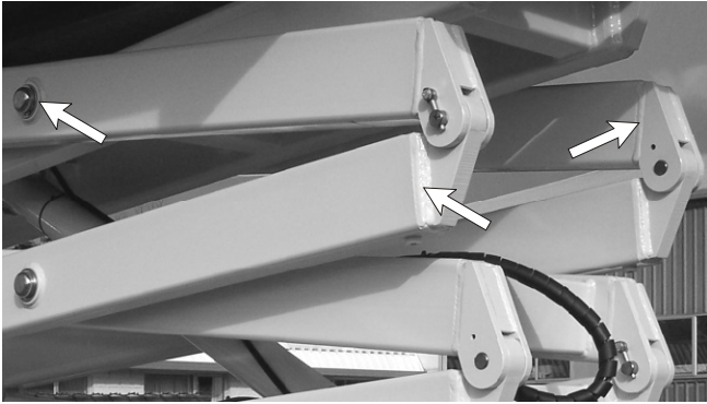
Figure 7.19 - Structural Damage and Welds
