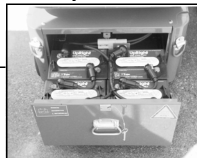
Figure 9: Access to Batteries
