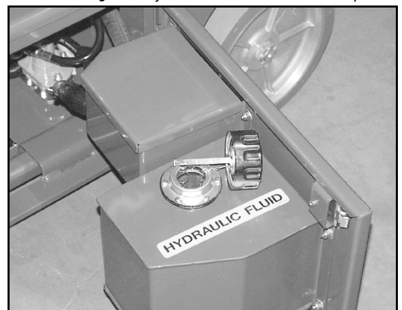
Figure 8: Hydraulic Fluid Reservoir and Dipstick
