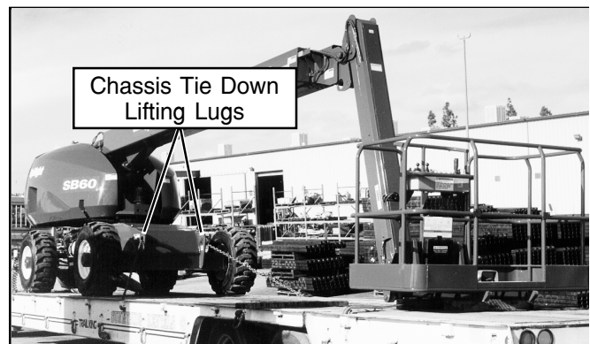
Figure 10: Rear chassis tie down lifting lugs.
