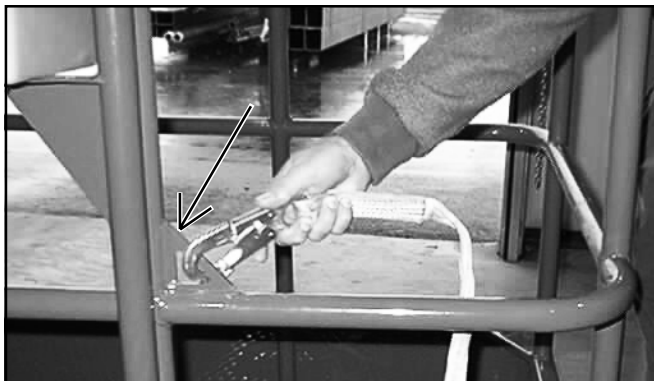
Figure 6: Typical Fall Restraint Anchorage Point
