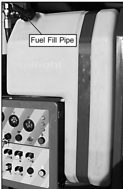
Figure 8: Fuel Fill Pipe
