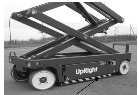
Pothole Protection Rails Lowered
