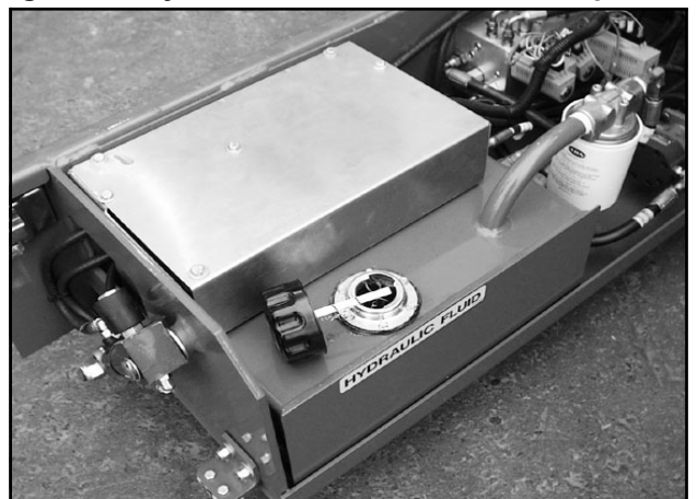
Figure 12: Hydraulic Fluid Reservoir and Dipstick
