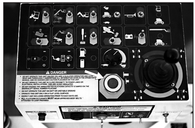
Platform control box Emergency Stop switch location.
