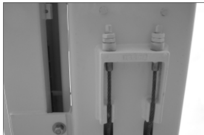
Figure 7.14 – Bottom of Main Boom at Tip End
