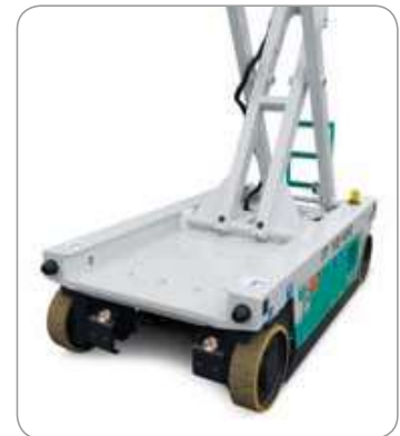
Functional chassis design for easy cleaning.
