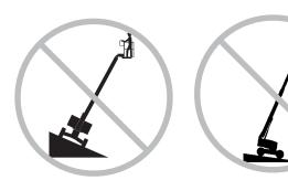
Do not raise or extend the boom unless the machine is on a firm, level surface.
