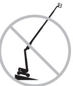
Do not depend on the tilt alarm as a level indicator. The tilt alarm sounds in the platform only when the machine is on a severe slope.
