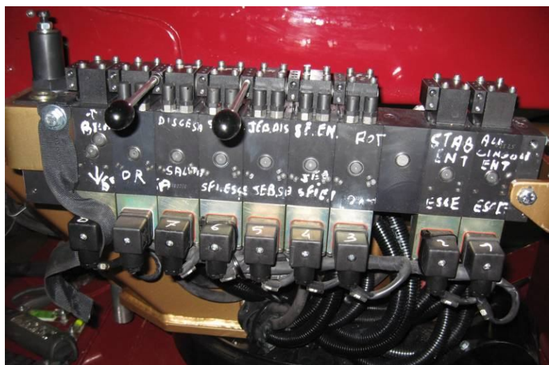
Hydraulic manual emergency controls in turret
